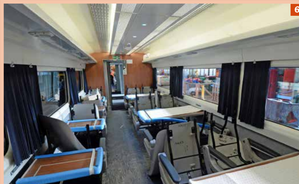
6. New leather First Class seats are yet to be fitted. The old seat arms and frames remain, but have been deep cleaned and repainted.
